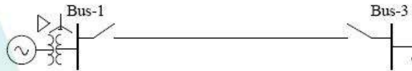
Fig. 14-5 Calculation of switching over-voltages on a transmission line.
